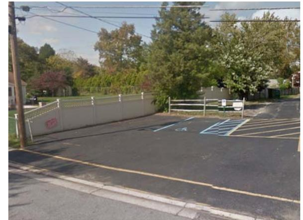
Parking spaces southwest and southeast of the post office can be replaced with pervious pavement to capture and infiltrate stormwater from the parking lot and rooftop runoff from the building. A preliminary soil assessment suggests that the soils have suitable drainage characteristics for green infrastructure.
