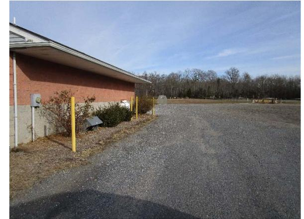
Parking spaces in the middle and northeastern parts of the lot can be replaced with pervious pavement to capture and infiltrate stormwater runoff from the remainder of the lot and rooftop runoff from the nearby building. A preliminary soil assessment suggests that the soils have suitable drainage characteristics for green infrastructure.
