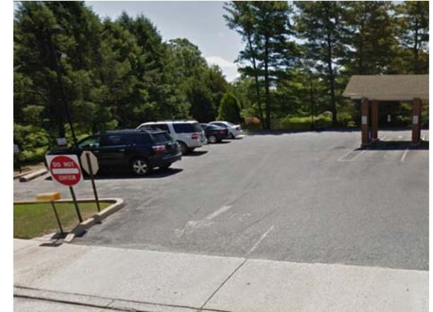
Parking spaces east and west of the bank can be replaced with pervious pavement to capture and infiltrate stormwater runoff from the remainder of the parking lot and rooftop runoff from the bank. A preliminary soil assessment suggests that more soil testing would be required before determining the soil's suitability for green infrastructure.
