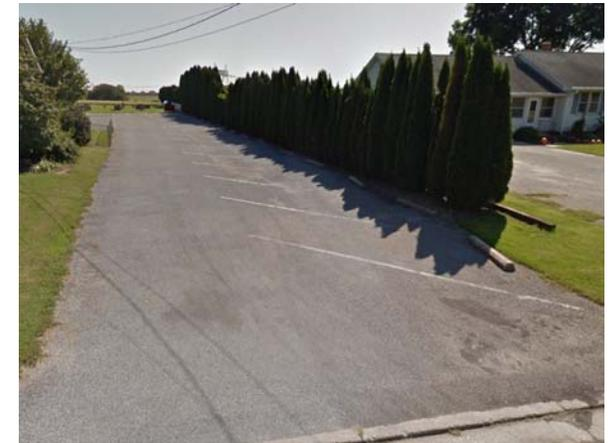
Parking spaces surrounding the church can be replaced with pervious pavement to capture and infiltrate stormwater runoff from the street and from the remainder of the parking lot. A preliminary soil assessment suggests that more soil testing would be required before determining the soil's suitability for green infrastructure.
