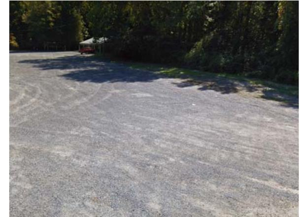
Southwestern parking spaces can be replaced with pervious pavement to capture and infiltrate stormwater from the street, from parts of the roof, and from the rest of the parking lot. Southeastern parking spaces can be replaced by pervious asphalt to infiltrate rooftop runoff from the remainder of the roof and parking lot. A preliminary soil assessment suggests that more soil testing would be required before determining the soil's suitability for green infrastructure.
