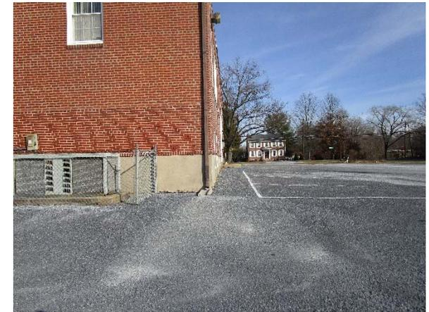
A stormwater planter can be installed along the west side of the municipal building to intercept and infiltrate roof runoff and to provide an aesthetically pleasing addition to the property. Pervious asphalt can replace the parking spaces alongside the northern and southern sides of the lot to capture and infiltrate runoff from the surrounding pavement. A preliminary soil assessment suggests that the soils have suitable drainage characteristics for green infrastructure.
